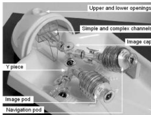
**Figure 2:** Dexter. Internal Components
