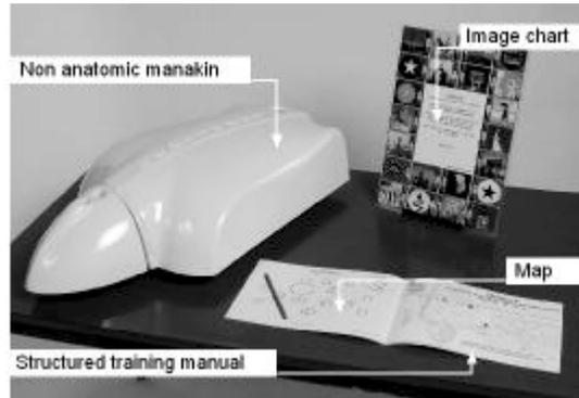
**Figure 1:** Dexter. An Endoscopic Dexterity Training System
