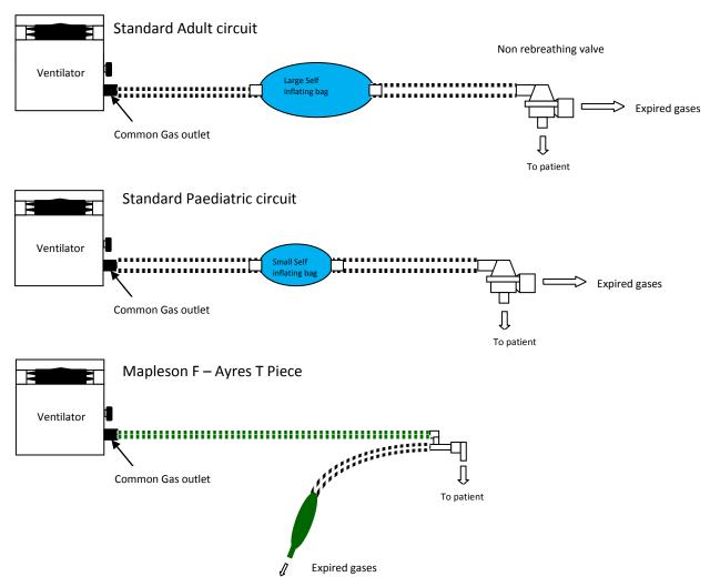
When using the Ayres T Piece the maximum pressure delivered can be set by adjusting the weights on the ventilator according to the scale. The pressure generated by the compression of the reservoir bag is displayed on the gauge on the ventilator. Flow rates for this circuit are usually advised as greater than 3 times the patient's minute volume. For paediatric patients, a mix of oxygen and air may be indicated, as high concentrations of oxygen (only) for long periods is contra-indicated.
