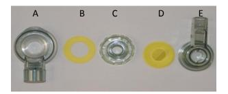
Part A will pull off from the valve The seal B can then be removed Part C can be unscrewed from part E The valve D can then be removed
