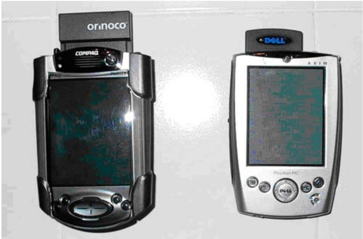
Figure 1: Compaq iPaq3900 and Dell Axim Handheld Computers with protruding external Network Interface Cards
